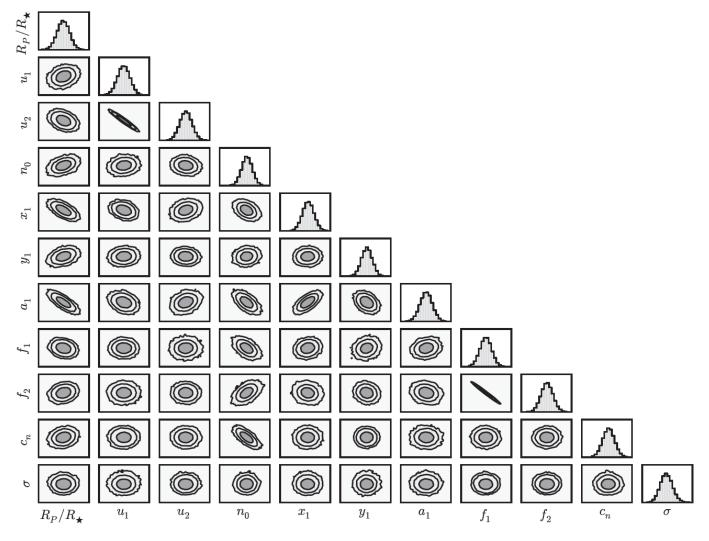
Fig. 14. Example correlation plots for the posterior parameter distributions for the fit of narrowband channel #9 (678 nm-698 nm). The lines indicate the areas encompassing  $1\sigma$ ,  $2\sigma$ , and  $3\sigma$  of the whole distribution, respectively.
