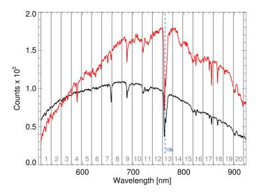
**Fig. 4.** Spectra of HAT-P-32A and reference star Ref2 from Run 2. Indicated in gray are the limits of the twenty 20 nm wide narrowband channels. The blue limit of the additionally defined 15 nm wide channel #13b excluding the first 5 nm of channel #13 is indicated with a blue dashed line.
