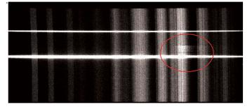
**Fig. 2.** Example of an image obtained in Run 1, which was contaminated by an internal light reflection. The image shows the light of HAT-P-32A (*bottom*) and the fainter reference star Ref1 (*top*) dispersed by the grism in the horizontal direction. The contaminating light reflection is indicated with a red circle.
