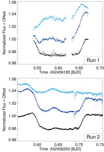
**Fig. 3.** Raw white light curves for HAT-P-32A (dark gray circles) and the reference star (light gray circles) for both observing runs and their division the relative white light curve (black circles). *Top panel*: data for Run 1, *bottom panel*: data for Run 2.
