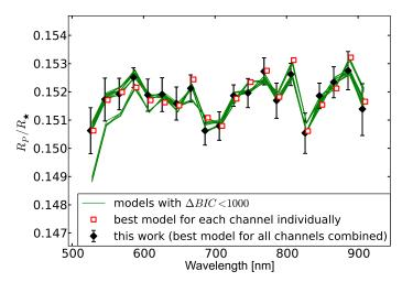
**Fig. 13.** Results for the wavelength-dependent, radius ratios obtained for the different models listed in Table 4 (green lines). The final adopted results, calculated with a homogeneous analysis, are overlayed as black diamonds (error bars are calculated as described in Sect. 6). The results obtained when using the individually best-suited model for each wavelength channel are plotted as red squares.
