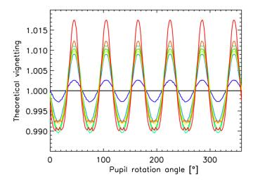
**Fig. 12.** Theoretical vignetting behavior as a function of effective pupil rotation angle derived from a simple toy model. The different colors represent different distances of the theoretically observed source from the telescope optical center (blue representing the closest distance and red the largest distance).
